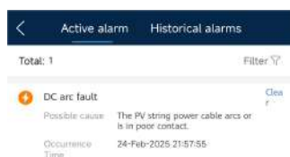
Figure 7-12 Clearing the alarm
