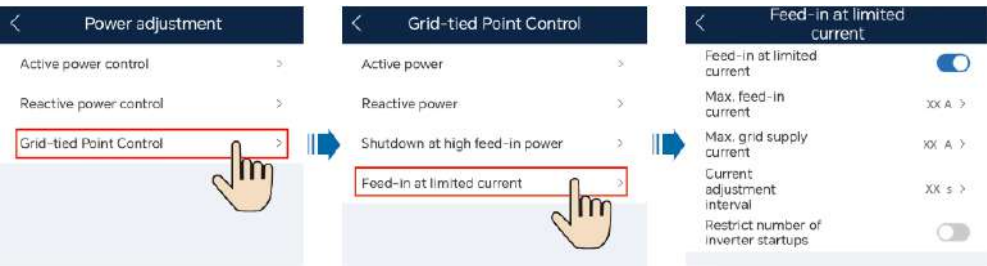
Figure 7-7 Feed-in at limited current
