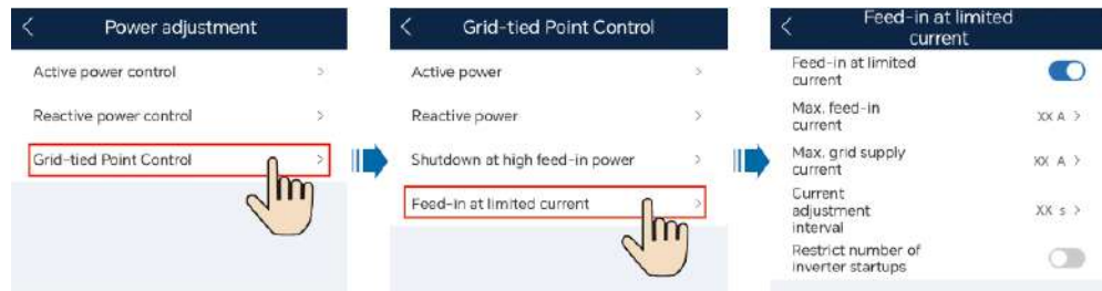
Figure 7-7 Feed-in at limited current
