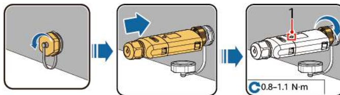
Figure 5-24 Installing the WLAN-FE Smart Dongle (WLAN communication)
